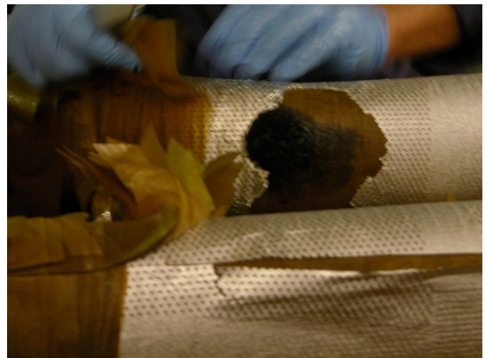
Fig. 1. The typical discovered defects after examination of unmounted transformers by producer.
