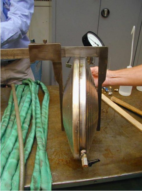
Fig. 2. Bellow distortion upon pressure feed of 5.5 bar.
