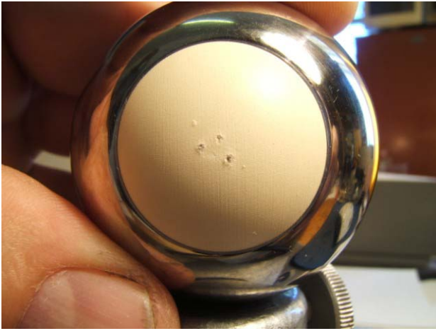
Fig. 2. Modified electrode. Dark spots show tracks of four previous discharges.
