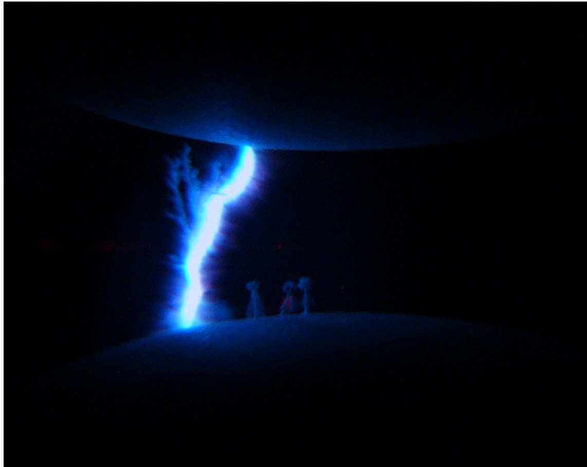
Near cathode – three nonelectrode streamers
