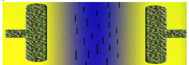
Figure 1. The pattern of the interelectrode gap with the conductive layers. Central blue zone is dielectric core, yellow near-electrode zone – conductive layers.
