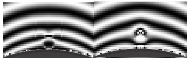
Fig. 8. Computed kerrograms (a) — single bubble on electrode, (b) — the same bubble after ionization.
