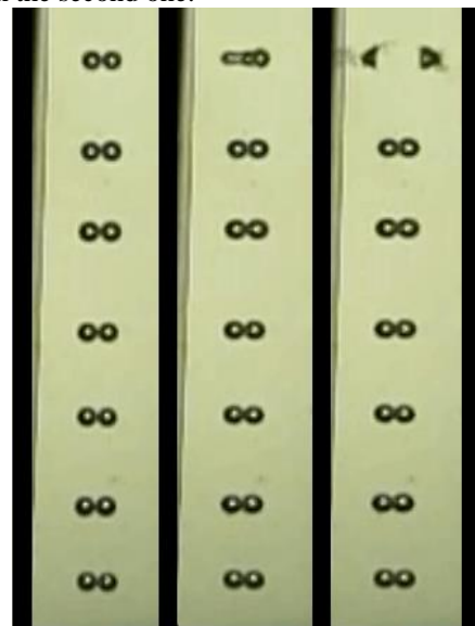
Fig. 4. Generation and floating of bubble's pairs.
