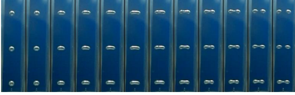
Fig. 5. Partial discharges in helium bubbles when exposed to x-rays. Voltage U=16 kV.
