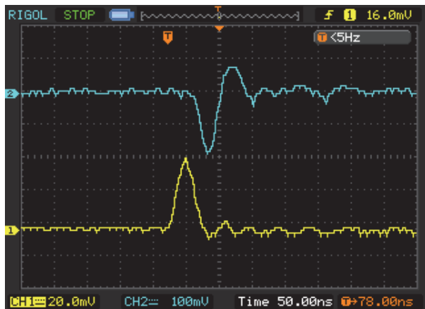
Figure 4. Signal from the partial discharge in a bubble of 1.7 mm diameter. Lower curve is the signal from the current transformer; upper one is from the registering circuit.
