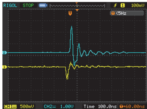
Figure 6. Signal from secondary PD. Lower curve is the signal from the transformer; upper one from registering circuit.
