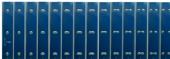
Figure 7. Partial discharges in helium bubbles when exposed to x-rays.
