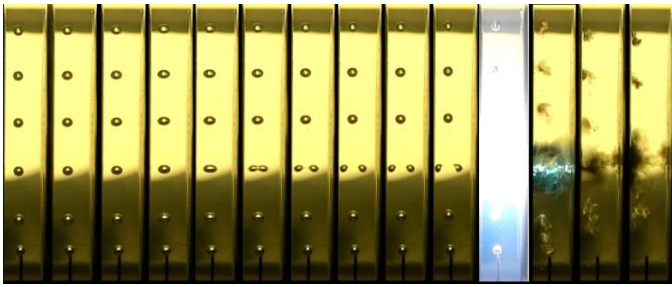
Fig. 7. Bubble dividing and following breakdown between bubble and electrode at E=3.3 kV/mm.
